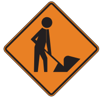
Work Crew Ahead
